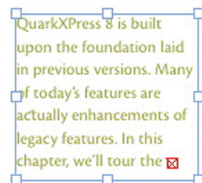
Figure 8 When you have more text than will fit in the box, an overset visual indicator appears like the one shown here.
